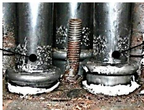
**Correct-** This tube is not overdriven. The flange has not bottomed out.
